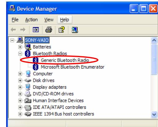
9. Switch to "Driver" tab in "Generic Bluetooth Radio Properties" windows and click "Update Driver" to replace the present Bluetooth driver by the installed BTW Bluetooth software.
