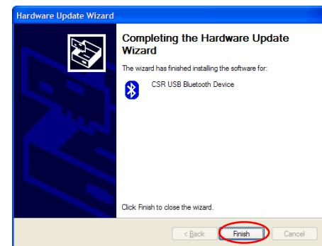
15. Open Windows "Device Manager" again, you will find out the "Bluetooth Device" instead of "Bluetooth Radio", and the device name is changed to "CSR USB Bluetooth Device".
